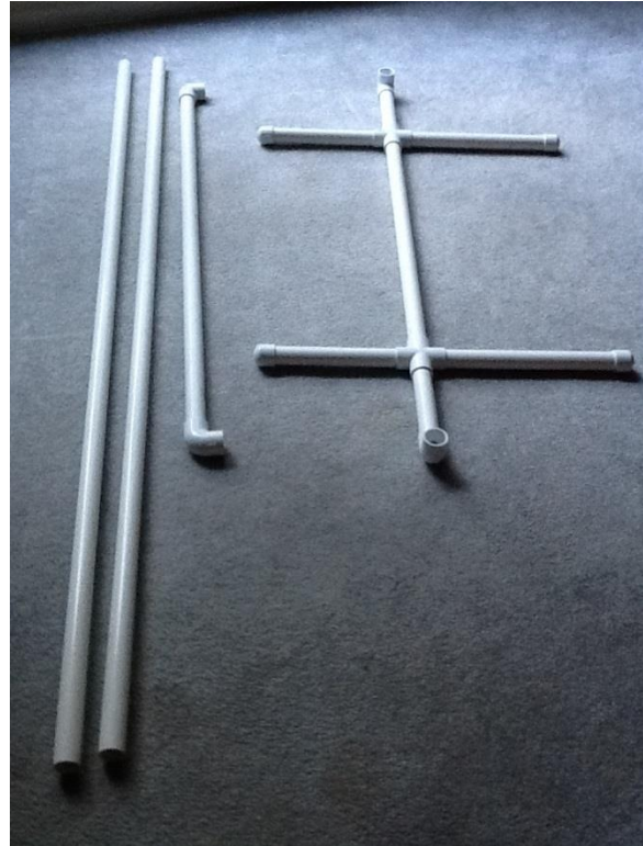
PVC components: 2 uprights, top bar, and base assembly
